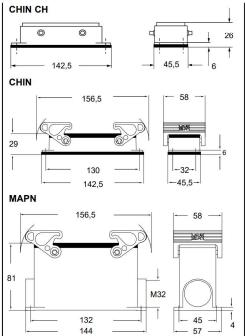
panel cut-out for bulkhead mounting housings CHIN CH and CHIN
