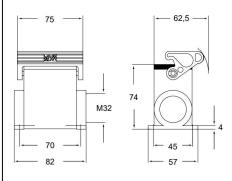
panel cut-out for bulkhead mounting housings CHIN LCH and CHIN L
