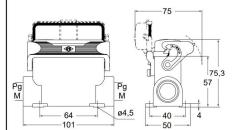
panel cut-out for bulkhead mounting housings
